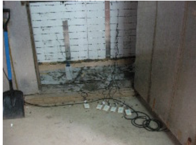
Installation of the Nomad temperature readers
